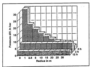
Fig. 3: Pressure distribution in the reservoir after the injection of the growth medium as a function of time and distance from the injection well.
